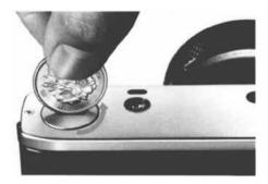
① Remove the cover of the battery chamber.
