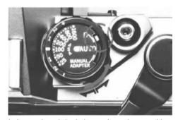
Indoors when it is dark, or when photographing at night, use the "BULB" setting and take the pictures by resorting to long exposures. Of course, blur can easily occur in long exposures so it is recommended to use a tripod and a cable release.
